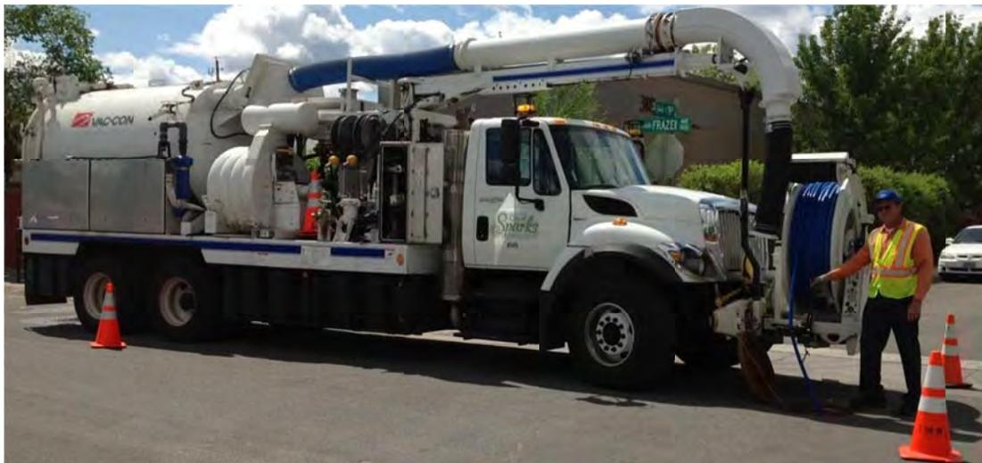
This larger capacity sewer maintenance truck saves time and ultimately money because of fewer trips to get water for cleaning and flushing activities. Additionally, this truck is ideal for cleaning sewer lines behind houses because of the extra-long 1,200 FT steel
