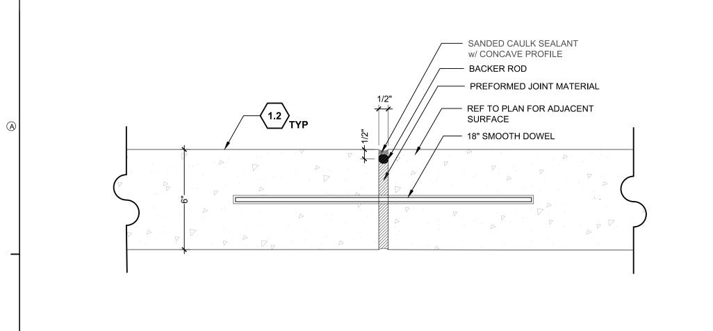
SANDED CAULK SEALANT w/ CONCAVE PROFILE - BACKER ROD - PREFORMED JOINT MATERIAL REF TO PLAN FOR ADJACENT SURFACE
