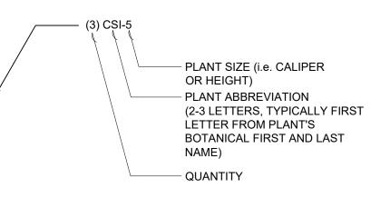
NOTE: PLANT ABBREVIATION ON PLANT IDENTIFICATION KEY SHOULD CORRESPOND WITH ABBREVIATION ON PLANT LIST (i.e. CSI-5 SHOULD REFER TO A CORNUS SERICEA 'ISANTI', 5 GALLON CONTAINER)
