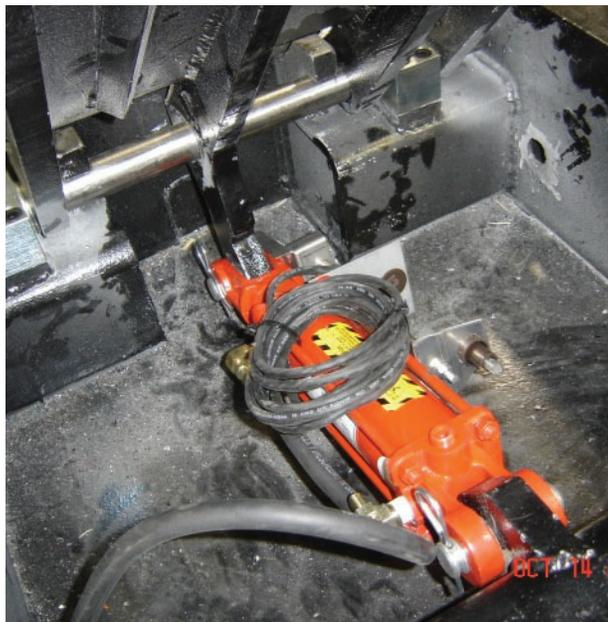
Photo 5 - Hydraulic cylinder installed for hoses to enter from the left, limit switch on right.
