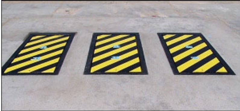
Photo 10 - The concrete has is cured and the protective covers have been removed. These units have been instrumented for the crash test.
