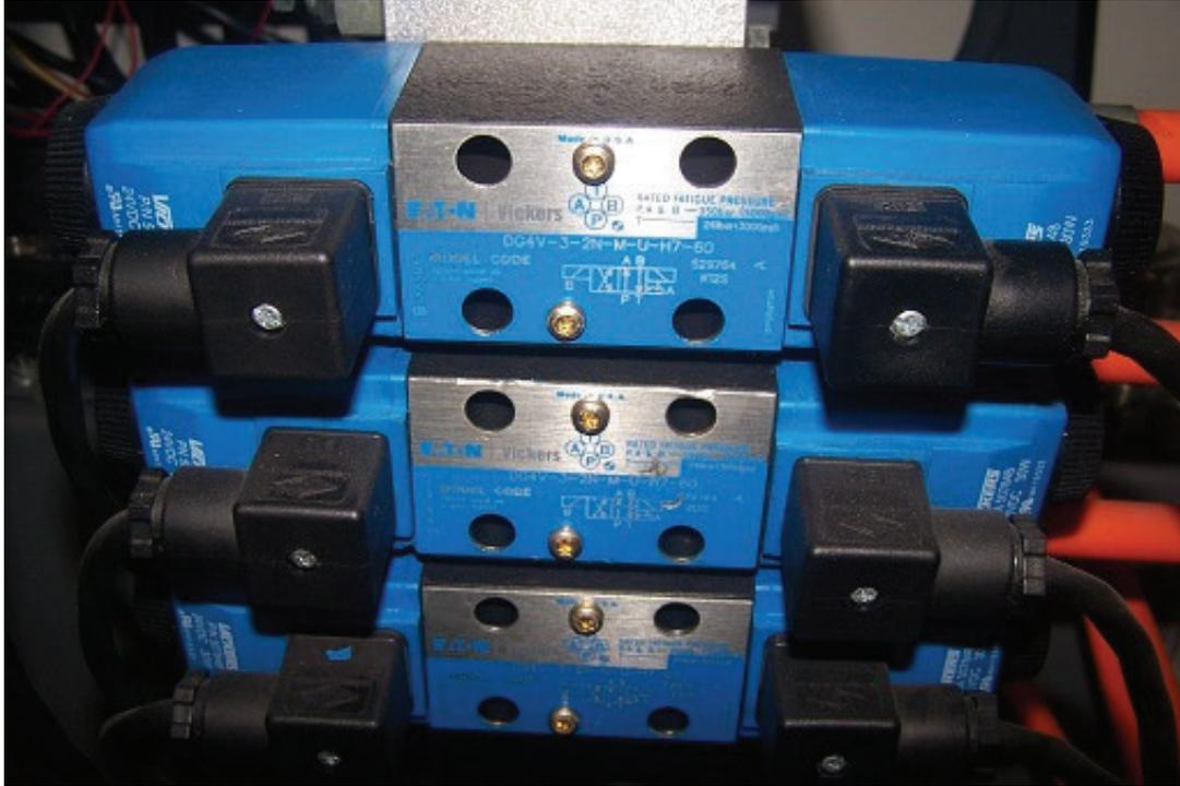
**Figure 3** – Vickers DG4V Directional valves mounted on manifold. Solenoids 'B' are on the left, solenoids 'A' are on the right.
