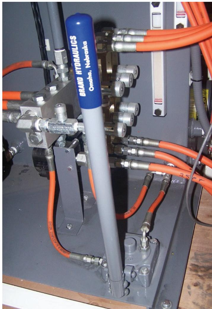
**Figure 5** – Manual hand pump. The pressure bleed down valve is mounted to the left of the hand pump handle.
