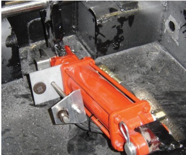
Photo 4 - Hydraulic cylinder installed for hoses to enter from the right, limit switch on left.
