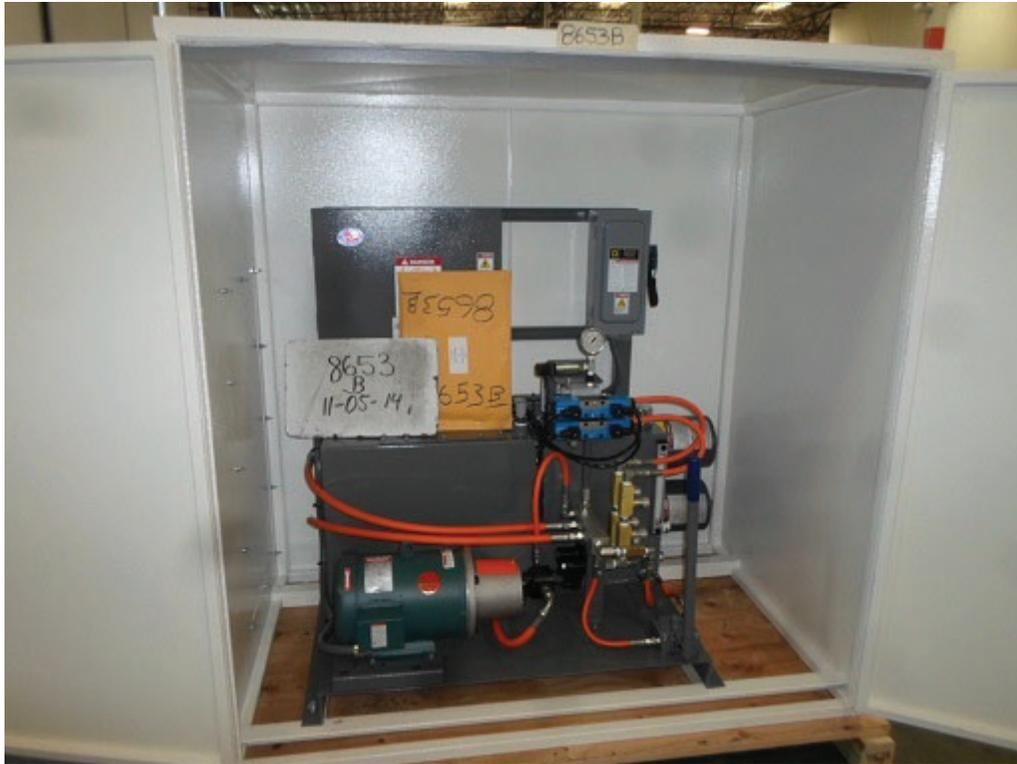
**Figure 1** – Typical Delta HPU mounted in enclosure.
