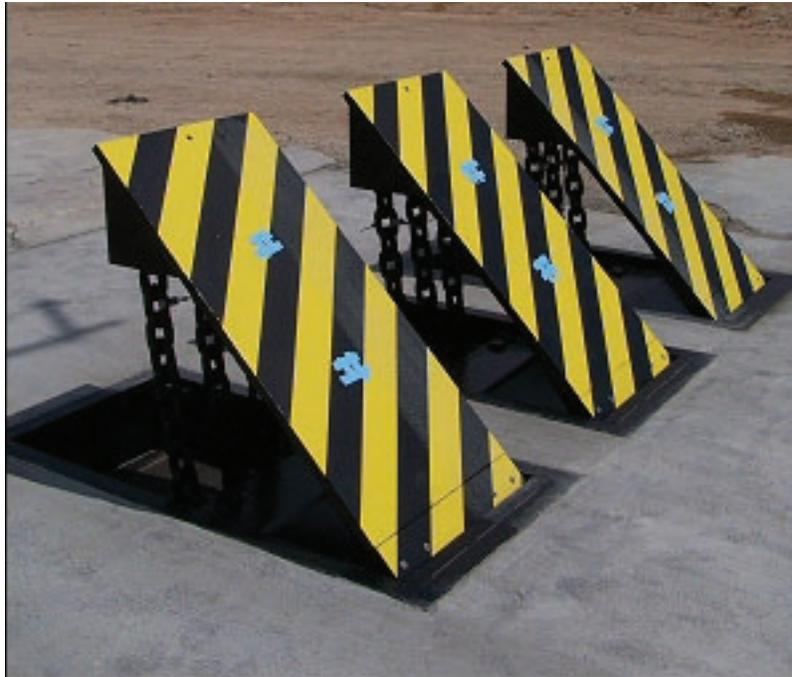
Photo 12 - Delta Model DSC2000 Phalanx in the guard position from the protected side. (The blue tape patches are to secure instrumentation for the crash test.)
