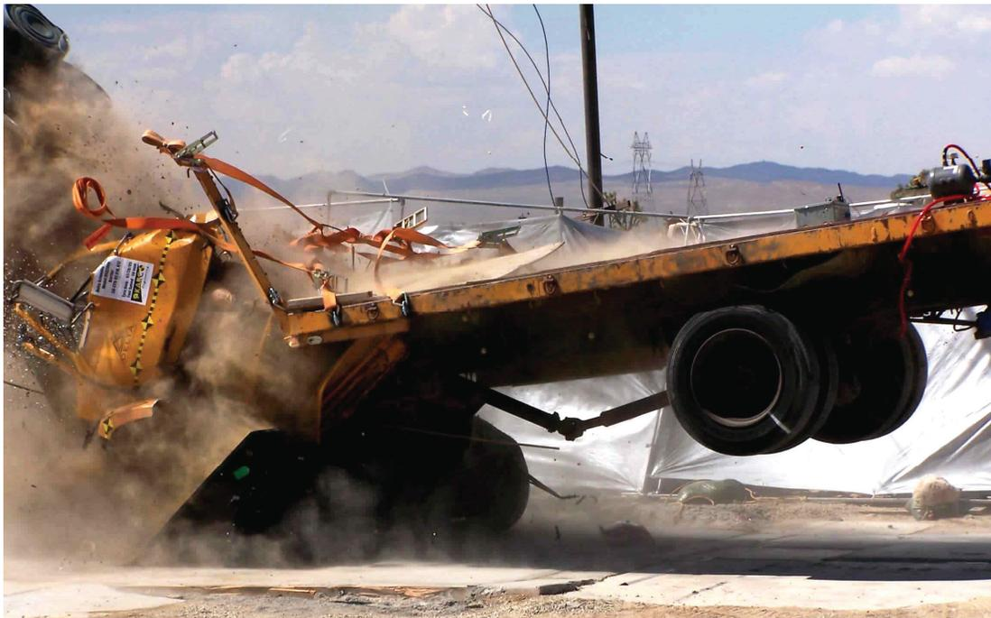
Photo 13 - Delta Model DSC2000 Phalanx at the moment of impact by a vehicle weighing 15,000 pounds [6,800 Kg] traveling at 50 mph [80 kph].
