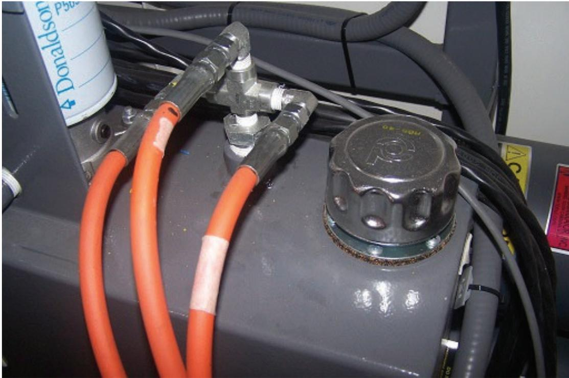
**Figure 7** – The cylinder rod vent hoses are terminated on fittings mounted on the reservoir tank top next to the oil filler breather cap and return filter.
