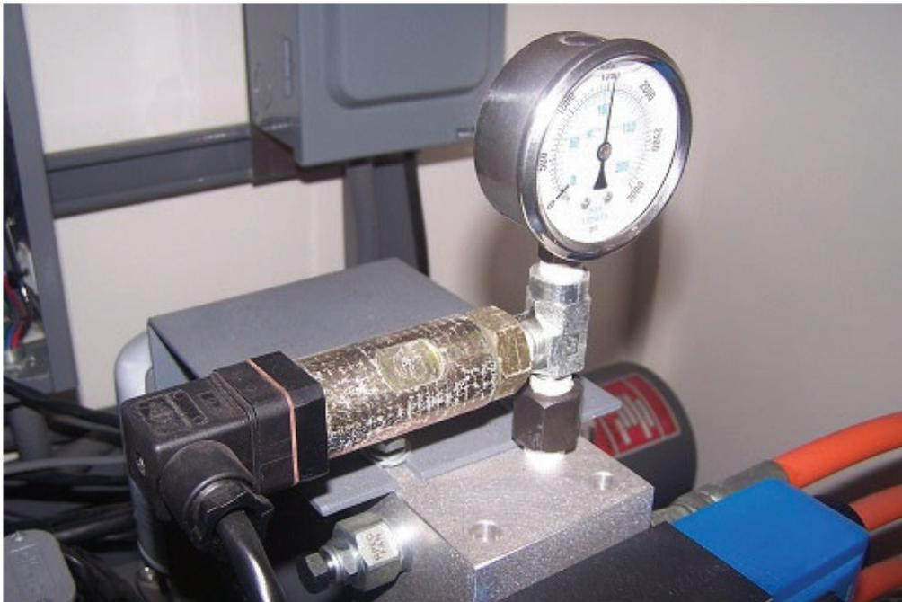
**Figure 2** – Pressure switch, pressure gage and pressure relief valve mounted on directional valve manifold.
