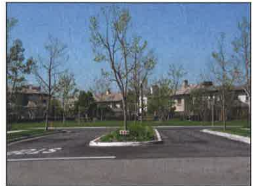
2.4.9 (a)(b) Raised planted medians calm traffic and pocket parks provide a neighborhood entry feature.
