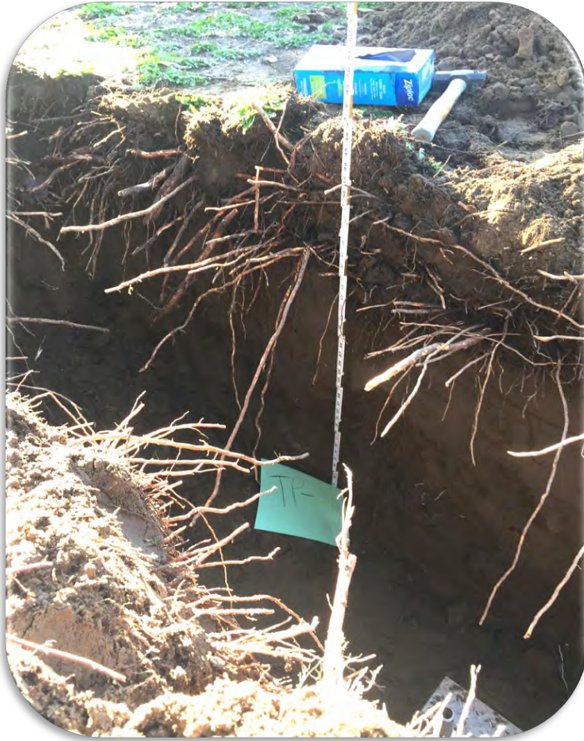
PHOTOGRAPH 2: Sidewall of TP-2. Note vegetation and root depths.
