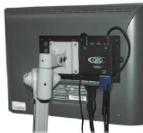
Remote unit mounted to the back of a flat panel monitor using ST-C5MK-VESA mounting kit
